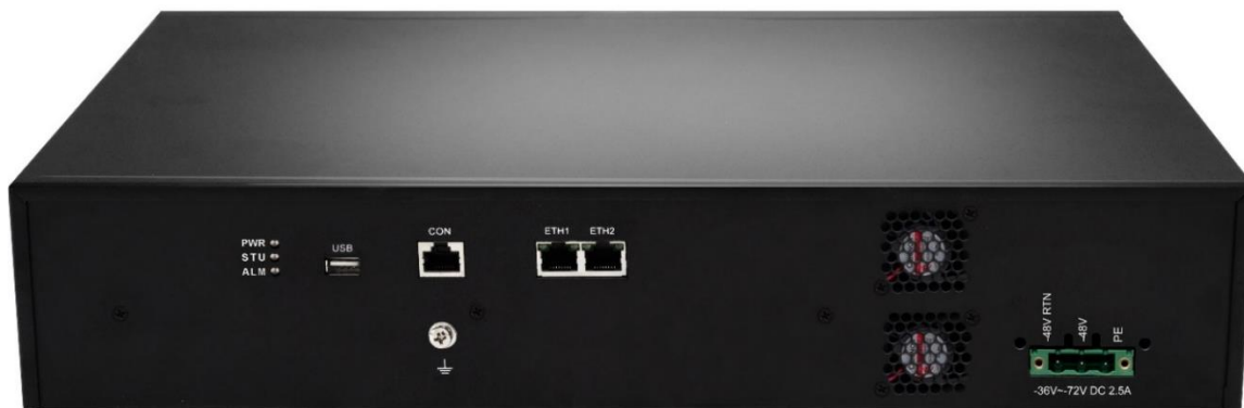
Figure 1-14 MX120 Back Panel-DC
