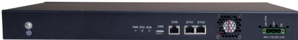
Figure 1-10 MX60 Back Panel-DC
