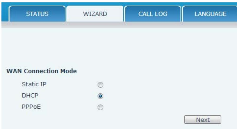
The connection mode of the phone varies with the network condition. You need to select a proper mode according to the real world situation. The NRP1012/P provides three network connection modes:
