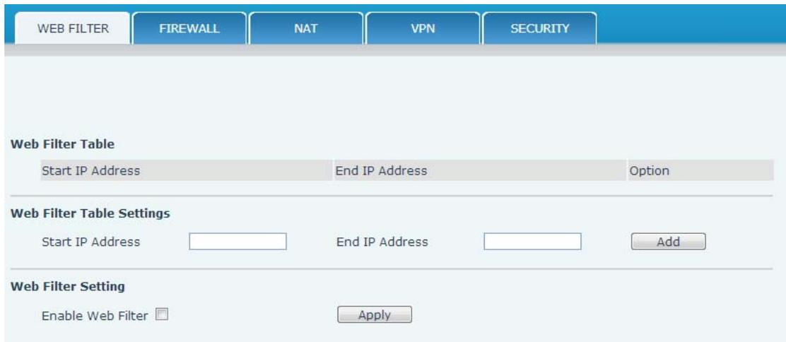
In this page, you can configure devices in a certain IP address segment to access the MMI of the phone for configuration and management.
